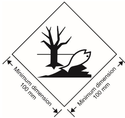
Environmentally hazardous substance mark
