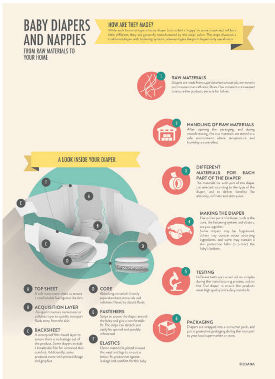
Figure 2 : Sectional diagram of a single-use baby diaper 12 (source : EDANA)
