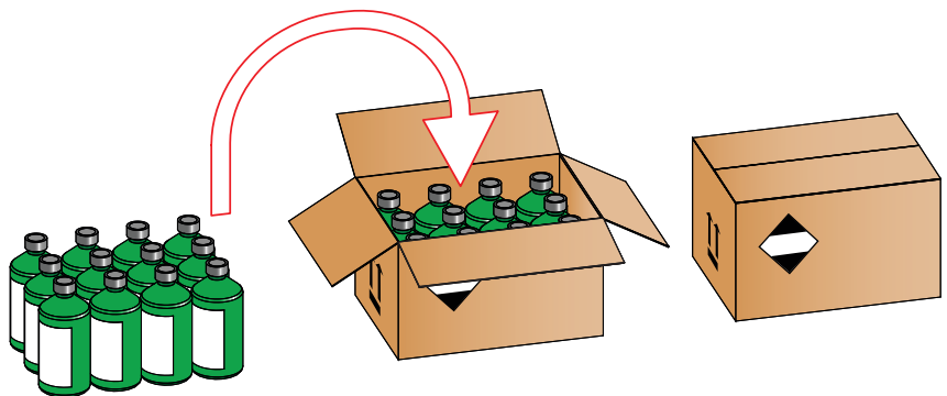
Construction of a typical combination package for dangerous goods: Separate inner packagings packed inside a fibreboard outer packaging
