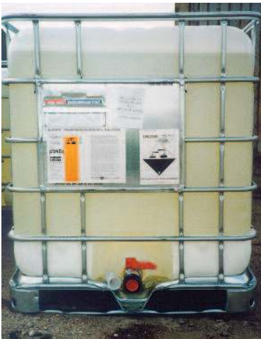
Typical rigid composite IBC
